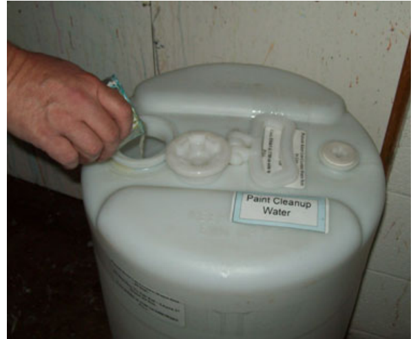
Pour the wash water into the provided drum
